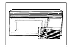
To replace your oven light, first disconnect power at main fuse or circuit breaker or pull plug.
